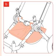
Attach the 2 hook and loop fasteners to the upper center shaft.
